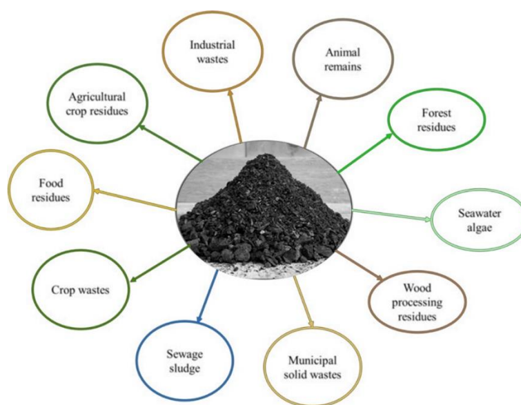
Figure 2. Various types of feedstocks used for the production of biochar (Content available from Biomass Conversion and Biorefinery )
